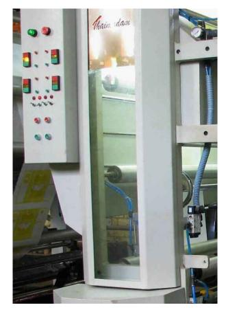
In the conventional machines, the operator has to sit down and look upwards, leaning inside the machine to get a view of the printed format or the doctor blade assembly if anything goes wrong the operator has to face a lot of troubles to get a clear picture of this situation. Almost all the upper area constituting drying chamber is enclosed and cannot be see from outside. This problem is completely eliminated in Thaimadam Machines.
