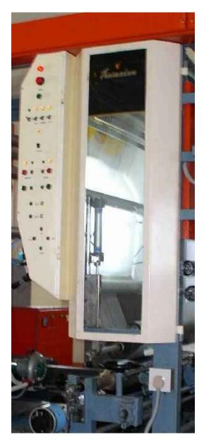
In the conventional machines, the operator has to sit down and look upwards, leaning inside the machine to get a view of the printed format or the doctor blade assembly if anything goes wrong the operator has to face a lot of troubles to get a clear picture of this situation. Almost all the upper area constituting drying chamber is enclosed and cannot be see from outside. This problem is completely eliminated in Thaimadam Machines.
